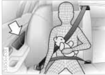
This is the right way a larger child should sit wearing the safety belt when rear side airbags (arrow) are installed.
