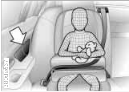
This is the right way a child should sit in a child restraint when rear side bags (arrow) are installed.
